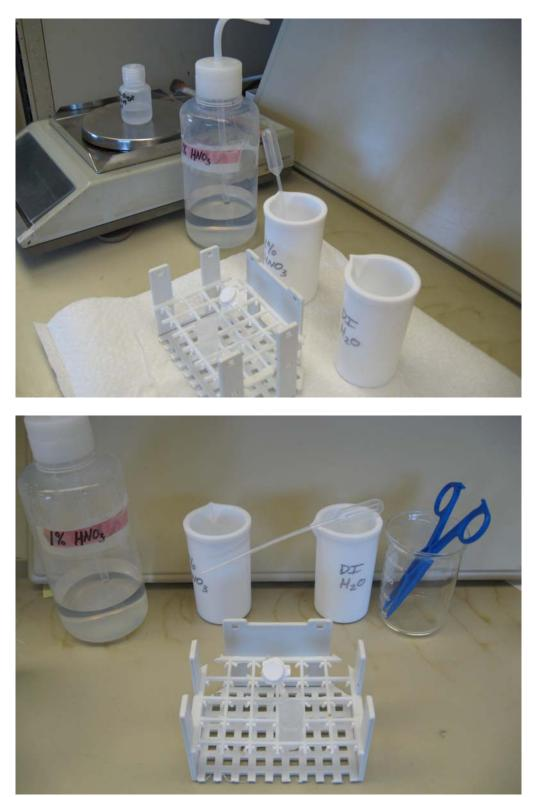
Preparation for transfer and dilution of mini peeper liquid to sample bottle.
