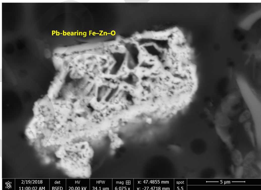
Figure I33. Pb-Bearing Fe-Zn-O Phase in Sample D-441-1B
