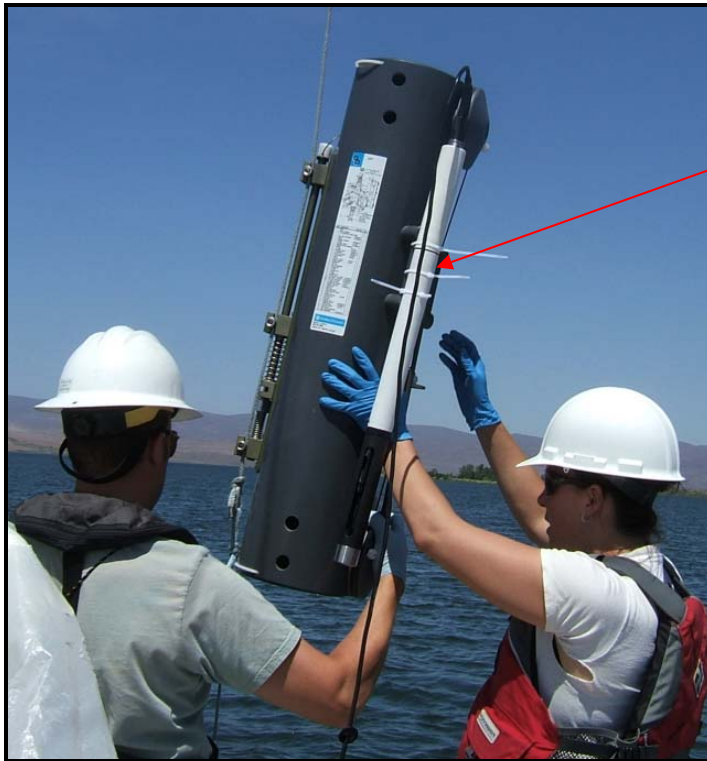
Figure 7. GO-FLO bottle with multiprobe attached to handle prior to deployment
