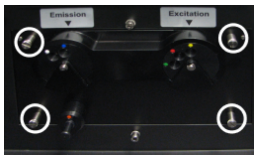
Figure 28: Filter change/Filter installation: Loosen the 4 screws
