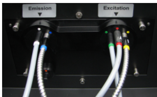
Figure 27: Filter change/Filter installation: First remove the optic (valid for all readers)
