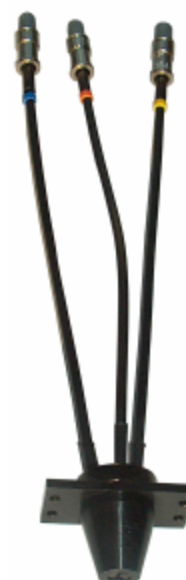
Figure 20: fluorescence polarization measurement head
