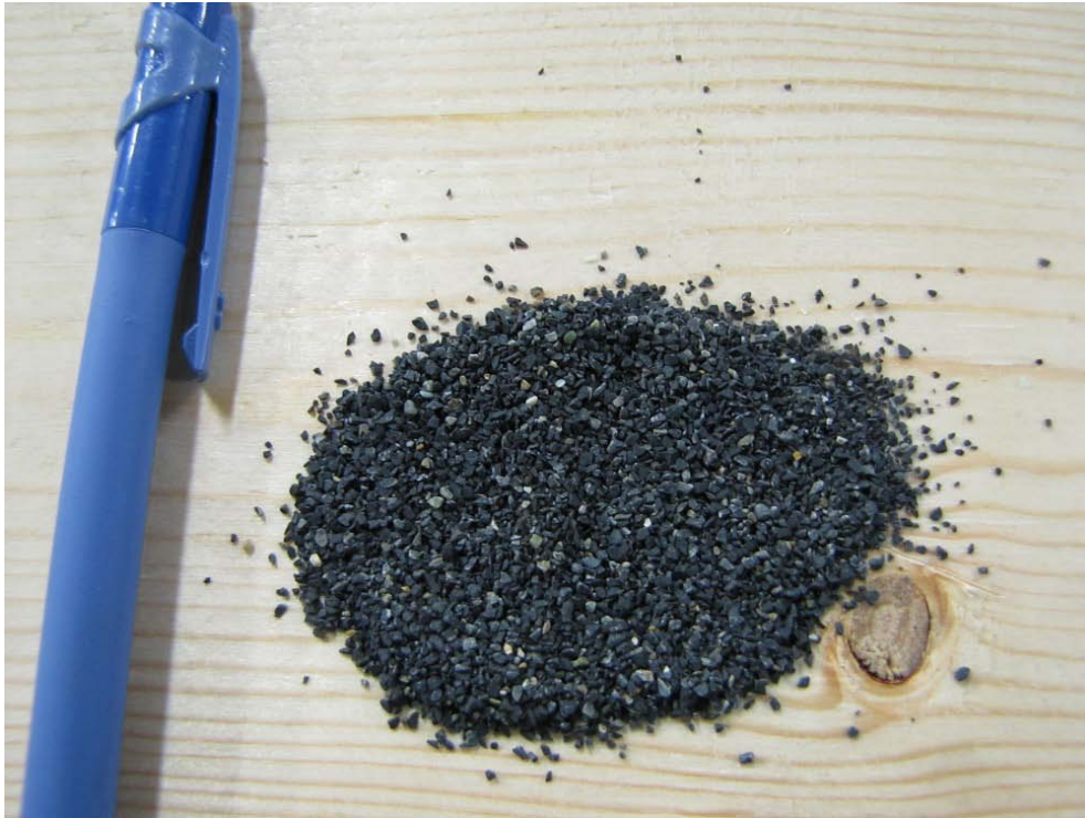
Figure 2.0 Hagen Geosystem Black Fine Gravel (ART# 12648) selected for further trials. Grain size of 0.85 to 1.68 mm with an average grain size of 1.11 mm. Dark coloration similar to UCR sediments.
