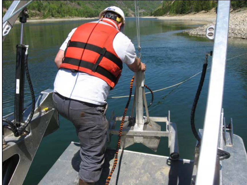
Figure 2 Deployment of the Power Grab sediment sampling device, Birchbank Eddy Station, view to the north.
