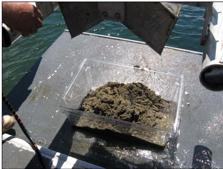
Figure 6 Sediment grab sample following placement in sample tray at the Genelle Station.
