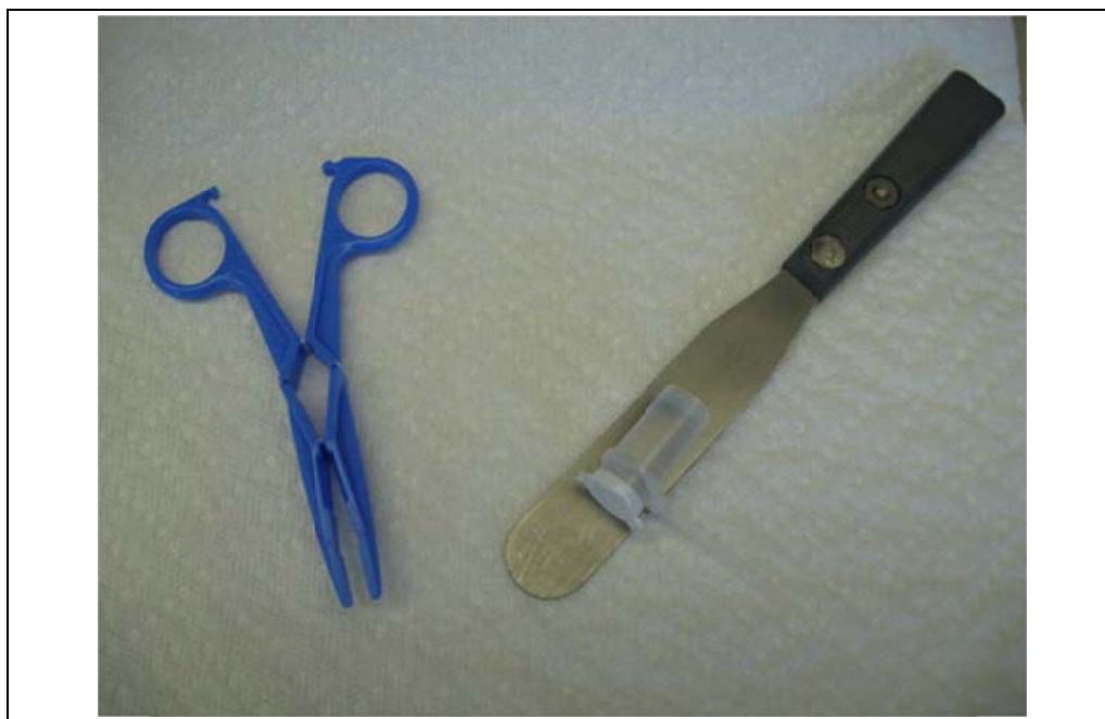
Photo 1. Typical tools for deployment of mini-peeper in laboratory test chamber
