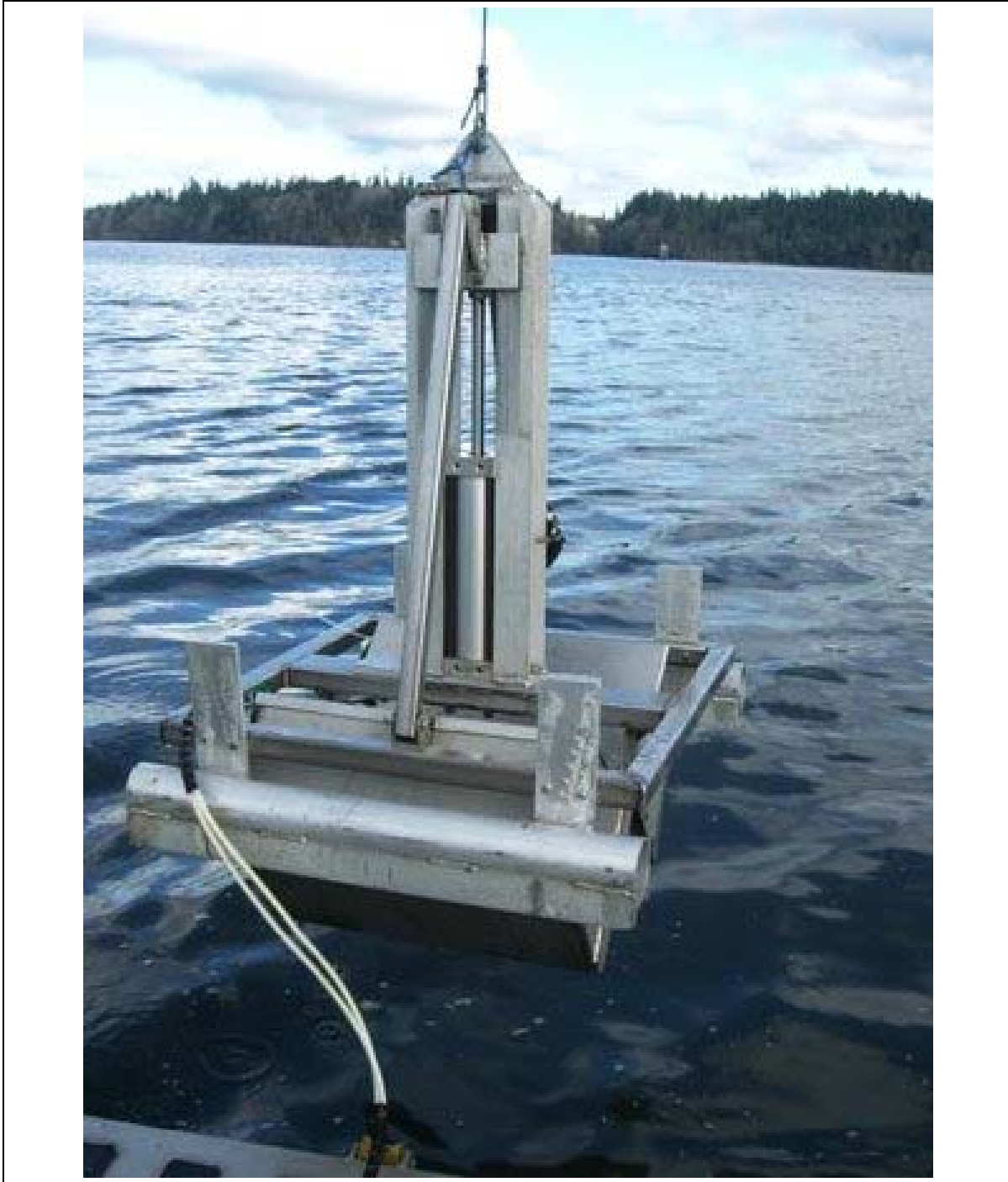
Figure 1. Illustration of Custom-designed Van Veen Power Grab Sampler
