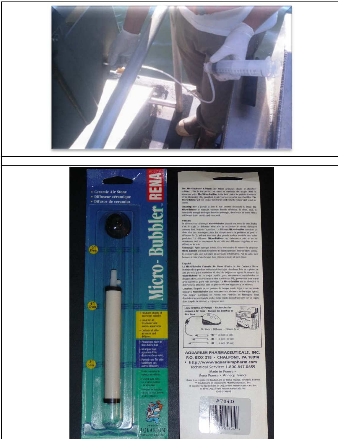
Figure 2. Illustration of Porewater Collection via Airstone and Typical Ceramic Airstone
