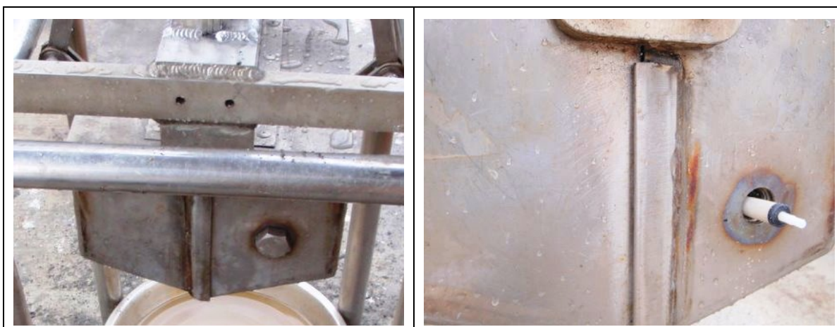
Figure A2. Illustration of Custom-designed Sampling Side Port on the Van Veen Power Grab Sampler
