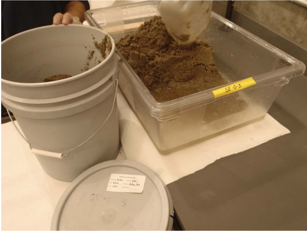
Homogenization of sediment consisting primarily of sand.
