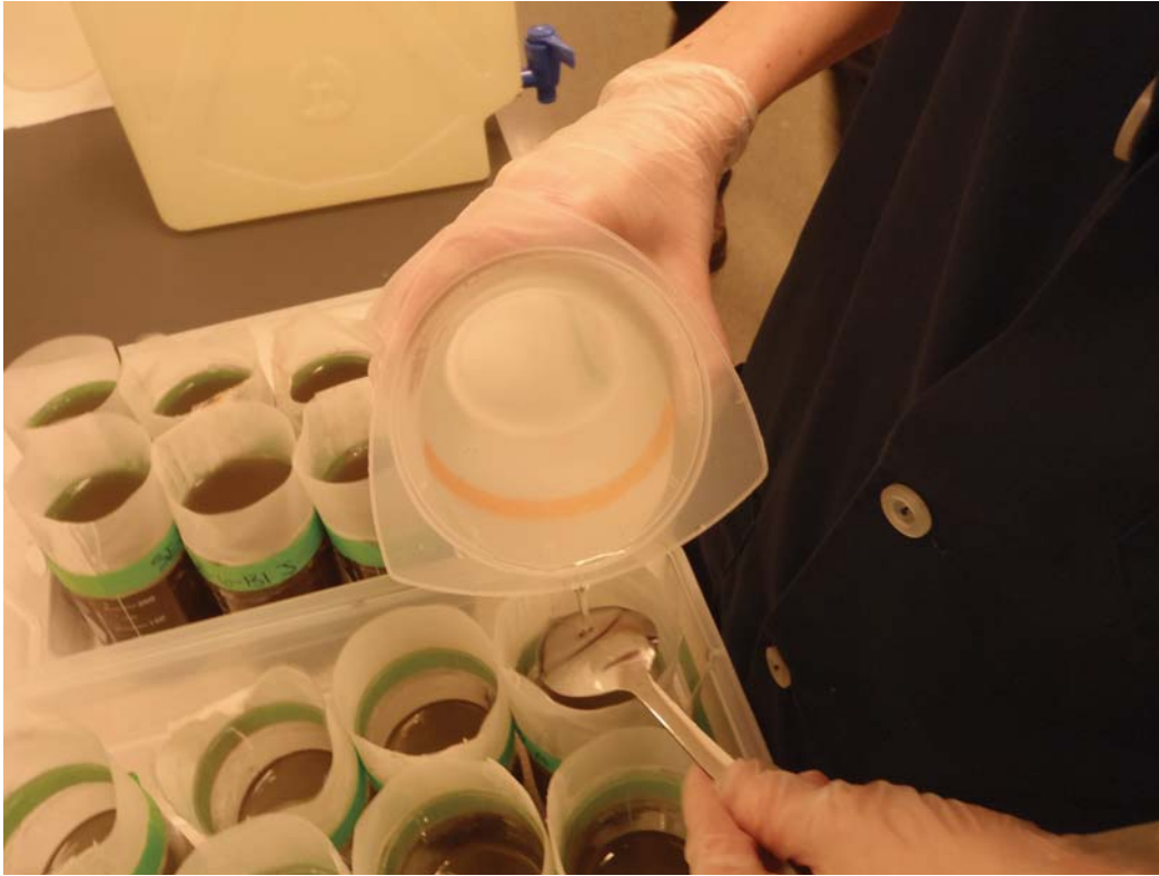
Addition of overlying water to test replicates at Day -1.
