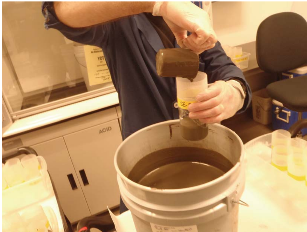
Loading "silt and clay" sediment into test replicate.
