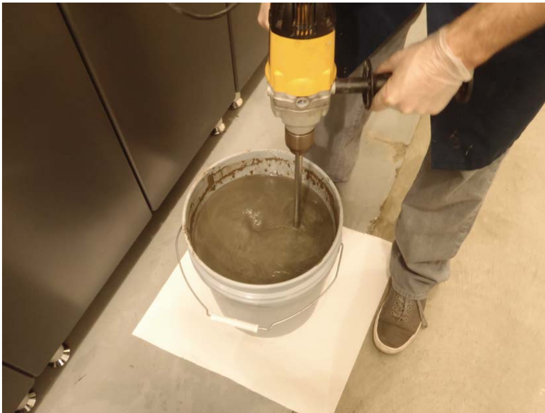
Homogenization of sediment consisting primarily of silt and clay.
