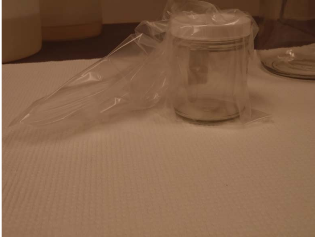
Demonstration of shipping and handling of AVS and SEM sample jars that cracked during freezing -Step 1: Jar placed in initial ziploc bag which is then purged with Nitrogen.
