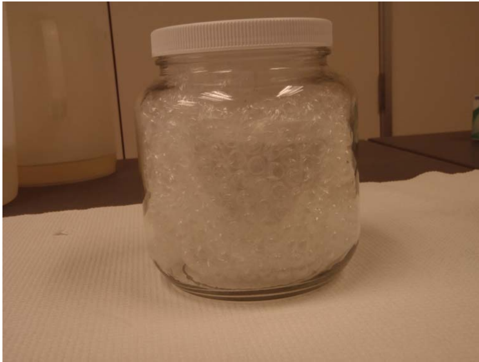
Demonstration of shipping and handling of AVS and SEM sample jars that cracked during freezing -Step 3: Bagged sample placed into 2-L jar, which is purged with nitrogen.
