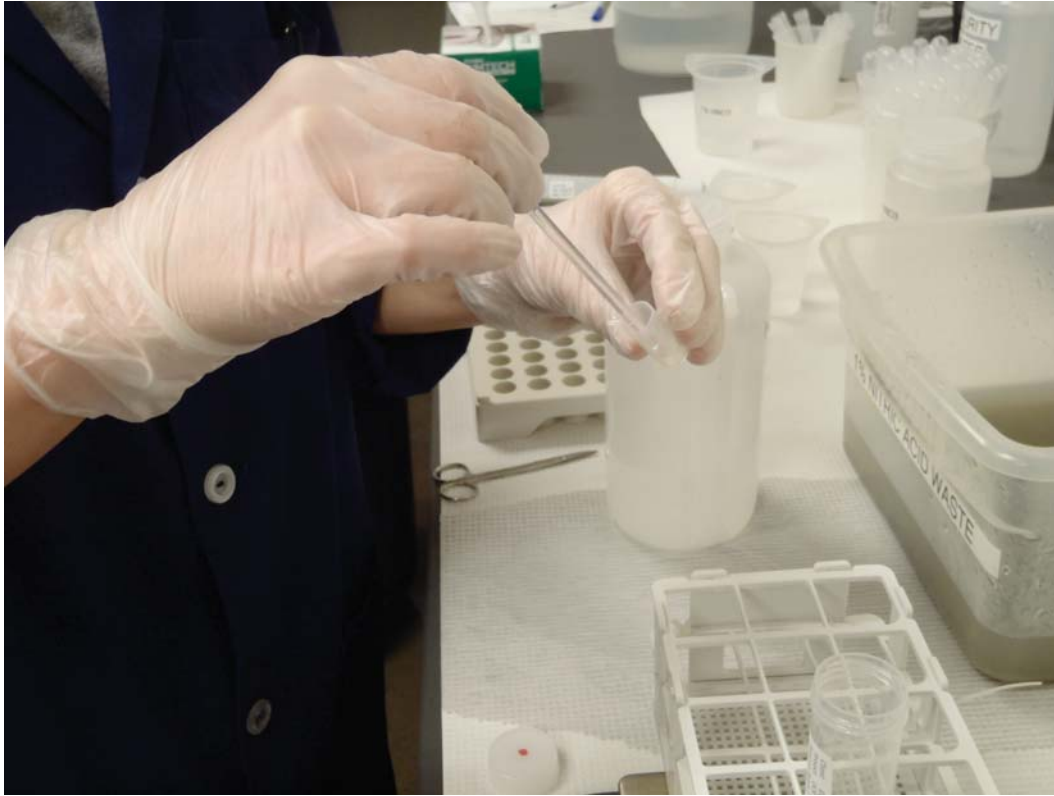
Collecting porewater sample from peeper.
