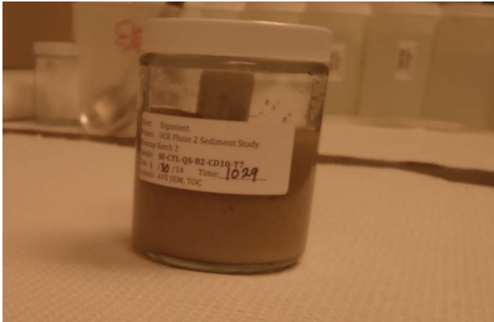
Example of AVS and SEM sample after addition of nitrogen gas.
