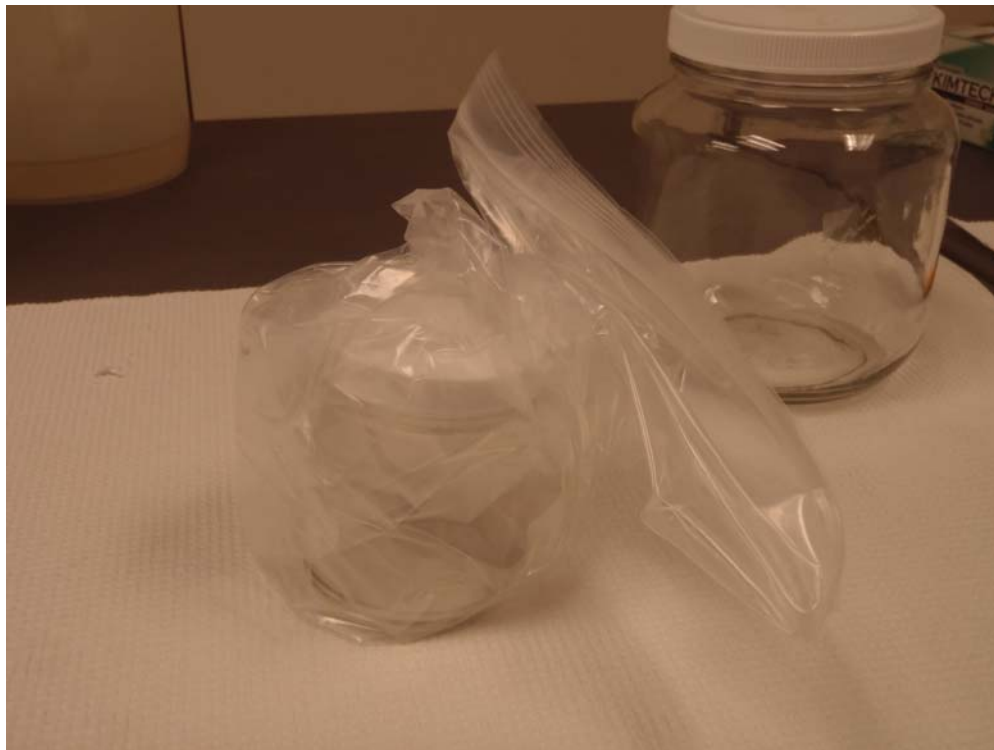
Demonstration of shipping and handling of AVS and SEM sample jars that cracked during freezing -Step 2: Jar and initial Ziploc bag placed into second ziploc bag which is also purged with nitrogen.
