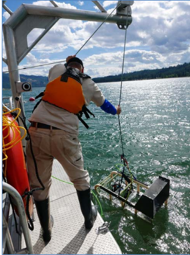
Photo 2: Underwater camera sled being deployed from the rear of RV Tieton.
