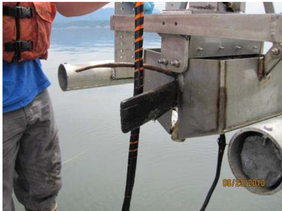
Wood debris and cobble in sampler at station LMF-03, sample attempt rejected.
