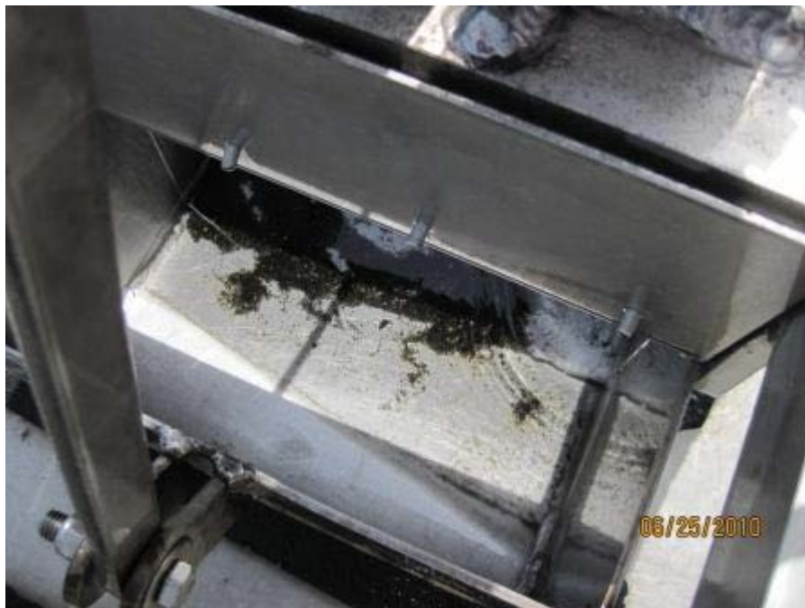
Sample washing and poor recovery at station CB- 02, sample attempt rejected
