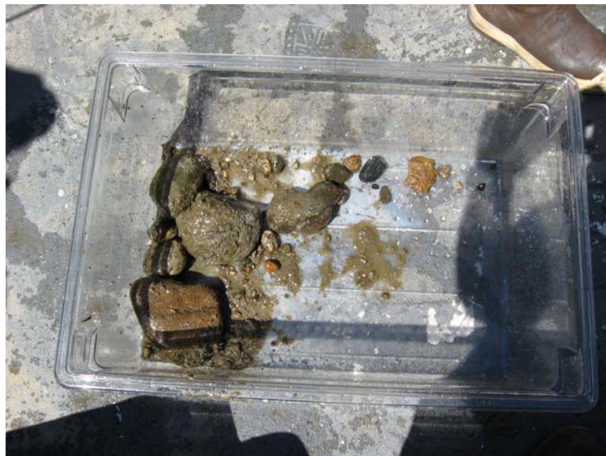
Figure 4 Poor recovery at Birchbank Eddy Station. Note cobbles and absence of finer sediment material.
