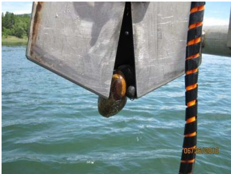
Gravels, cobbles and boulders in sampler at station DME-01, sample attempt rejected
