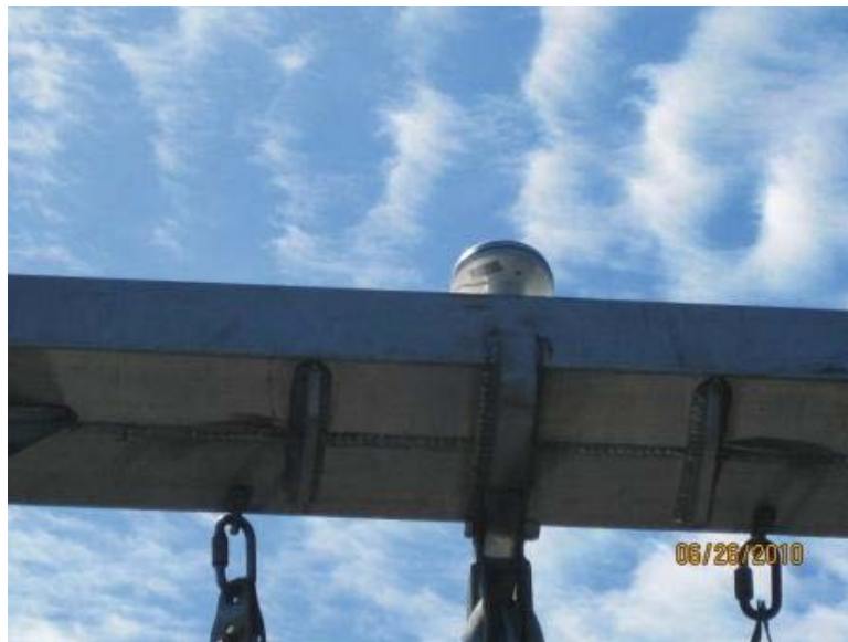
Nobeltec™ antenna located on top of forward boom over the Power Grab Sampler
