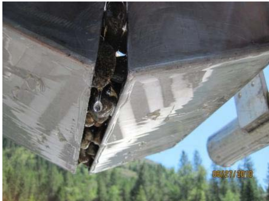
Gravels and cobbles blocking sampler at station LD-02
