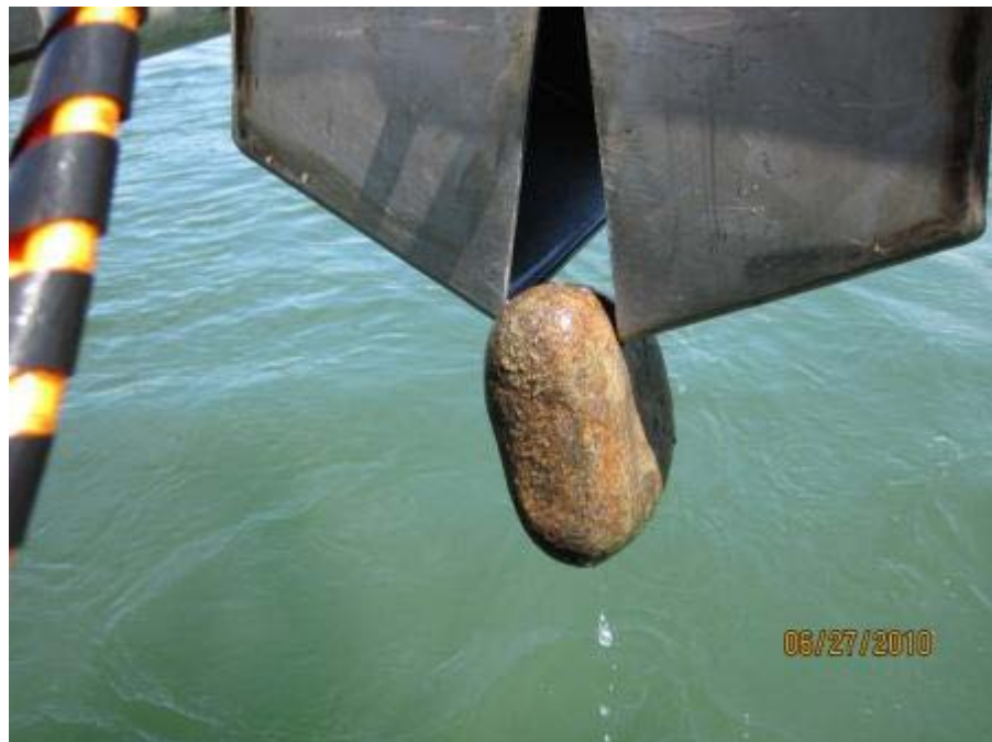
Boulder in sampler at LD-03, sample attempt rejected
