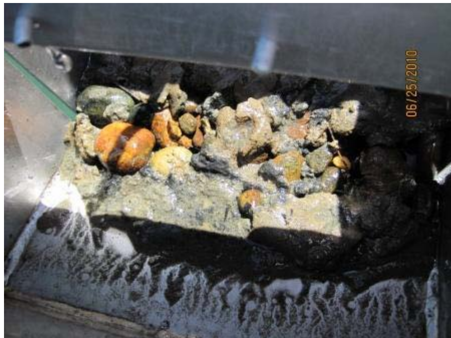
Gravels and cobbles blocking sampler with sample washing at station CB-03, sample attempt rejected
