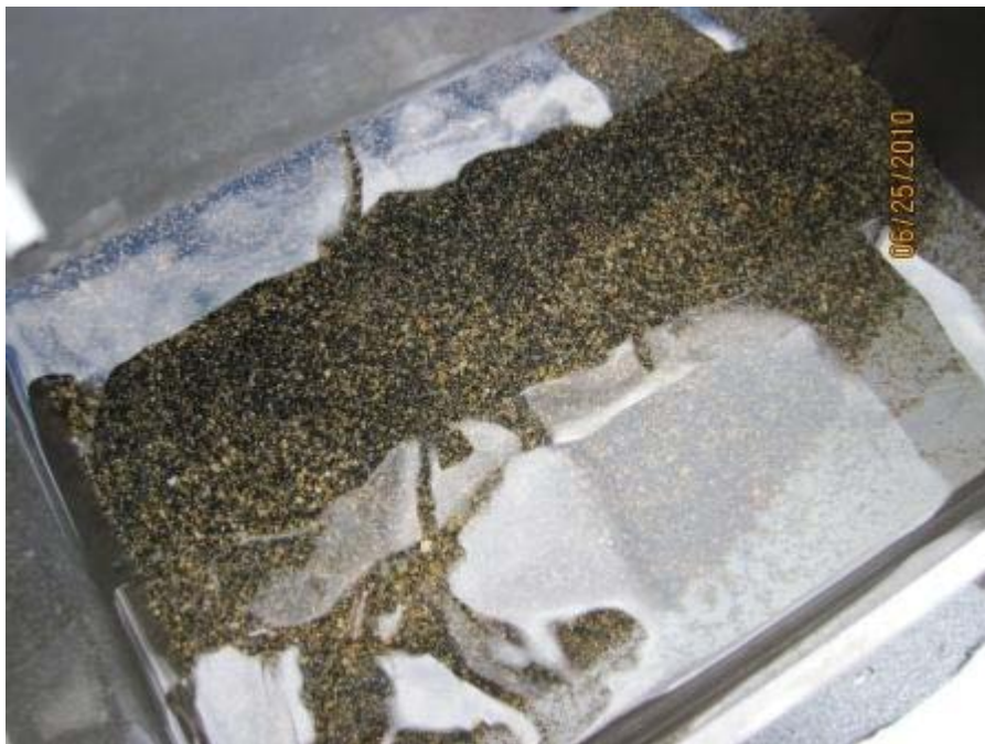
Sample washing and poor recovery at station CB-01, sample attempt rejected
