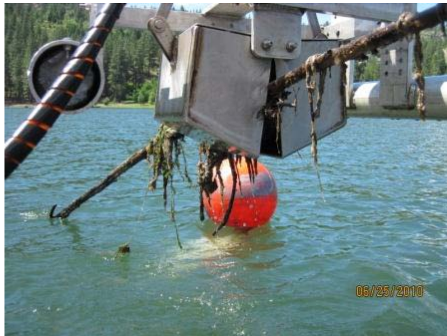
Wood debris in sampler at station CB-03, sample rejected
