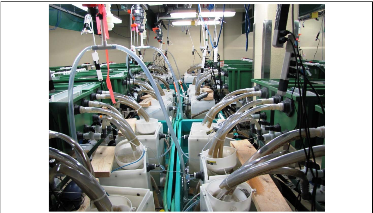
Photo D-6. White sturgeon sediment toxicity test exposure chambers as set-up at the University of Saskatchewan, Aquatic Toxicity Research Facility. Close-up of dedicated recirculating systems employed for each sediment exposure chamber duration of the study.
