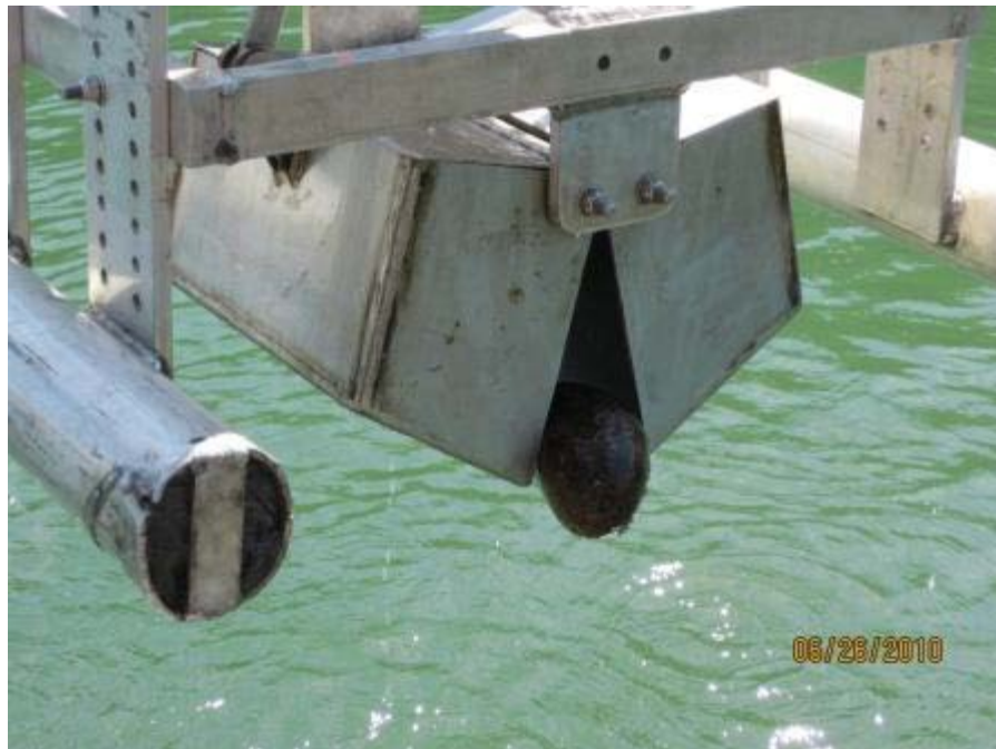
Boulder in sampler at station DME-02, sample attempt rejected
