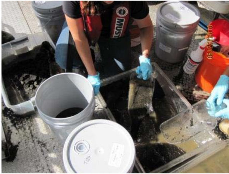
Sediment sample transfer from Lexan tub to 5-gallon HDPE container
