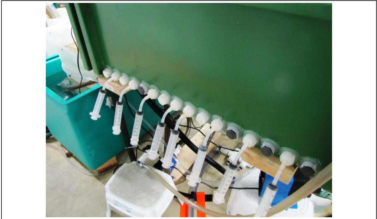
Photo D-7. White sturgeon sediment toxicity test exposure chambers as set-up at the University of Saskatchewan, Aquatic Toxicity Research Facility. Close-up of dedicated porewater extraction portals for ceramic airstones employed for the duration of the study.
