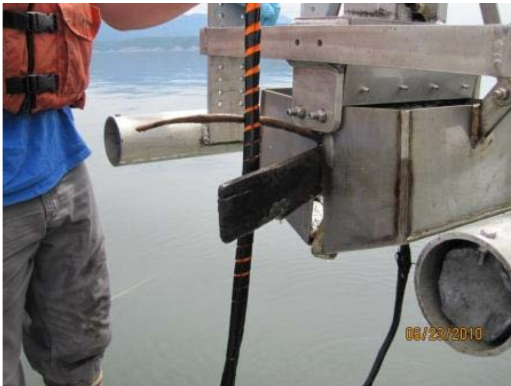
Photograph 5. Cut lumber and cobble in sampler at station LMF-03.
