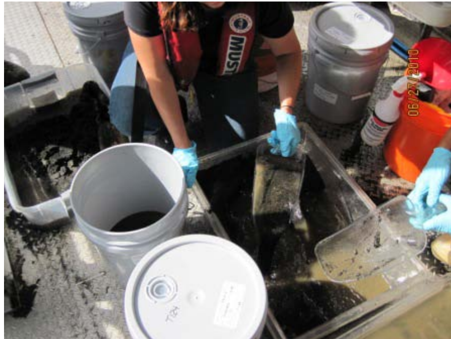
Transferring sediment sample to the 5-gallon HDPE containers
