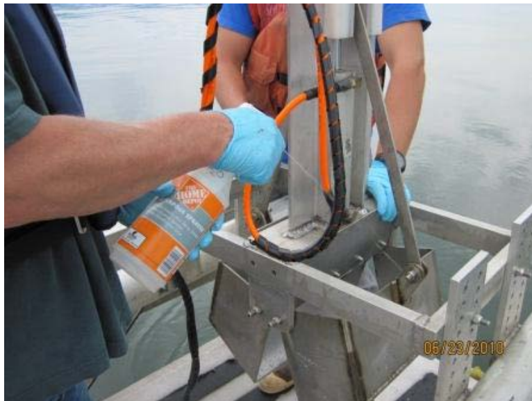
Decontamination rinse of the Power Grab Sampler using de-ionized water
