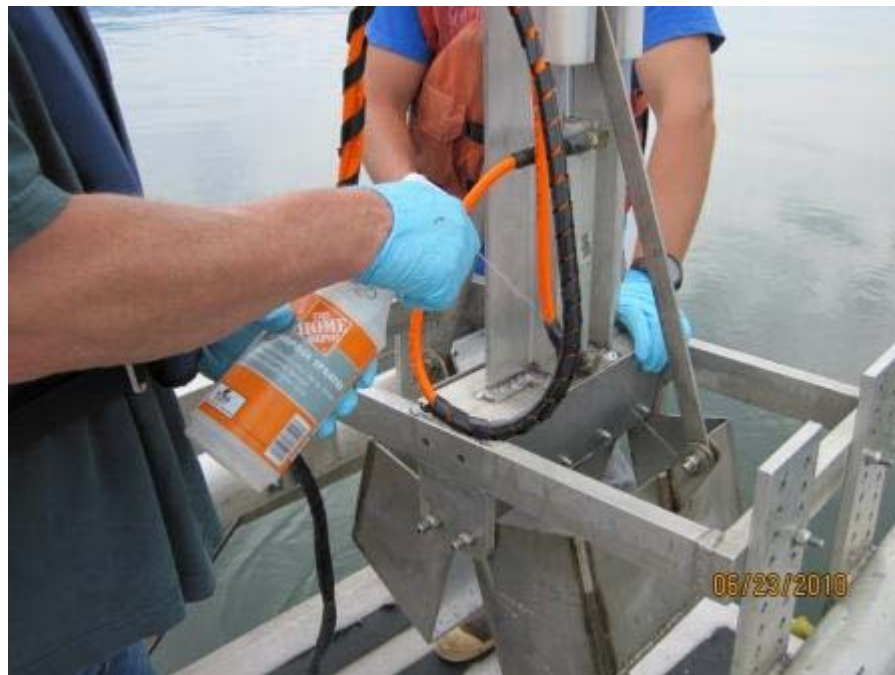
De-ionized water rinse step of Power Grab Sampler decontamination
