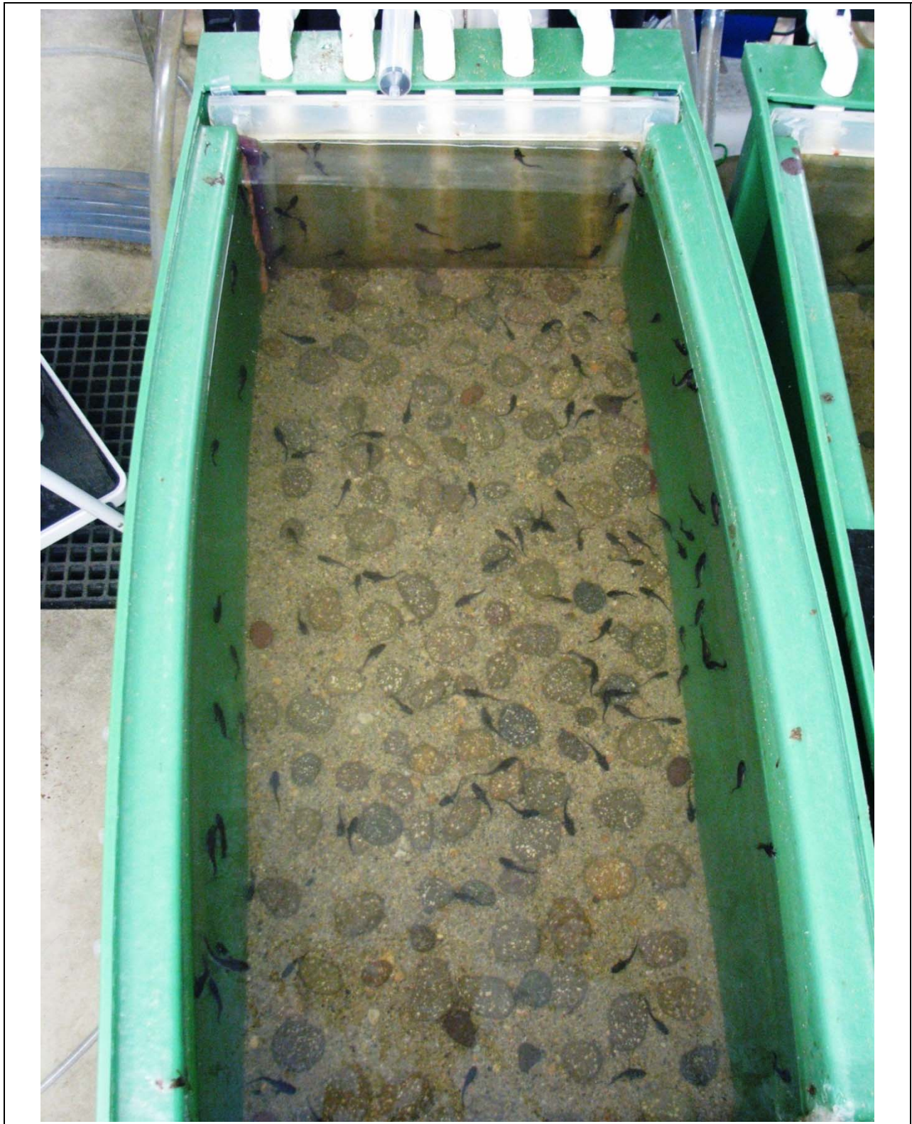
Photo D-8. White sturgeon sediment toxicity test exposure chambers as set-up at the University of Saskatchewan, Aquatic Toxicity Research Facility. Close-up of sediment exposure chamber containing white sturgeon as employed for the duration of the study.
