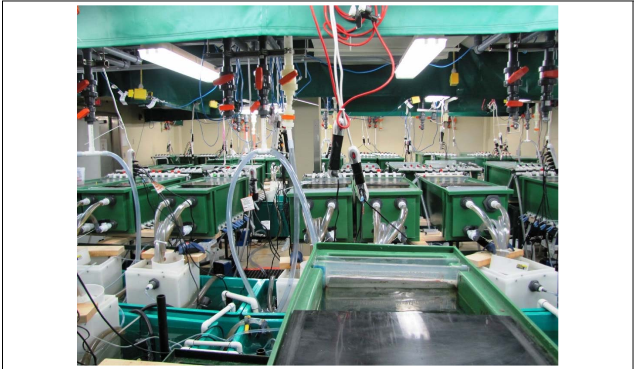
Photo D-3. White sturgeon sediment toxicity test exposure chambers as set-up at the University of Saskatchewan, Aquatic Toxicity Research Facility. Each green tub represents an exposure chamber.
