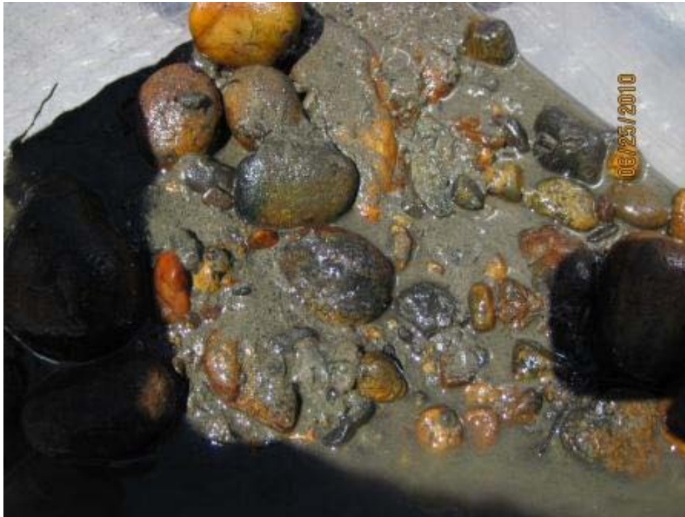
Photograph 6. Sample washing and poor recovery at station CB-03.
