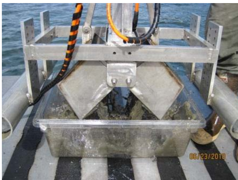
Lowering the Power Grab Sampler onto the boat deck and release of sediment into Lexan tub
