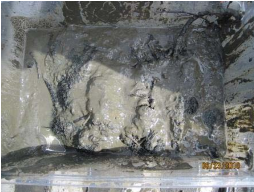
Wood debris in sample preventing closure of sampler, sample attempt rejected
