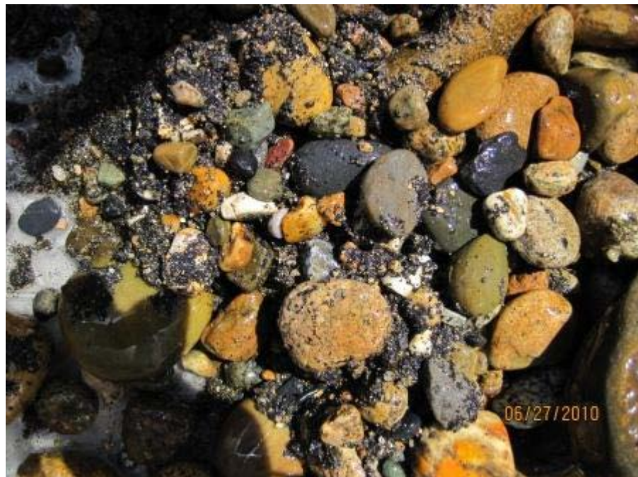
Sample in Lexan tray at LD-02, sample rejected due to sampler blocking and washing
