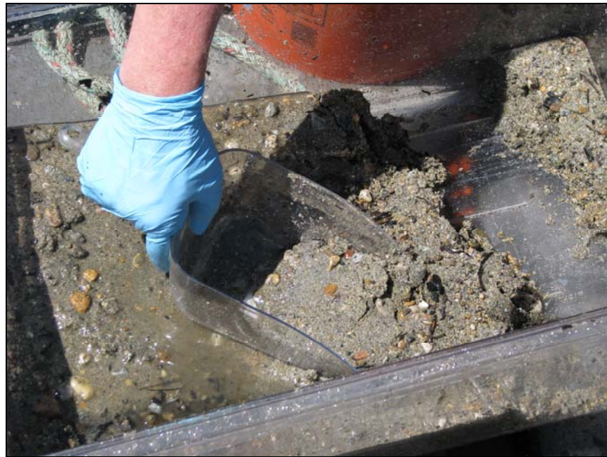
Figure 8 Transferring Genelle Station sediment grab sample from sample tray.
