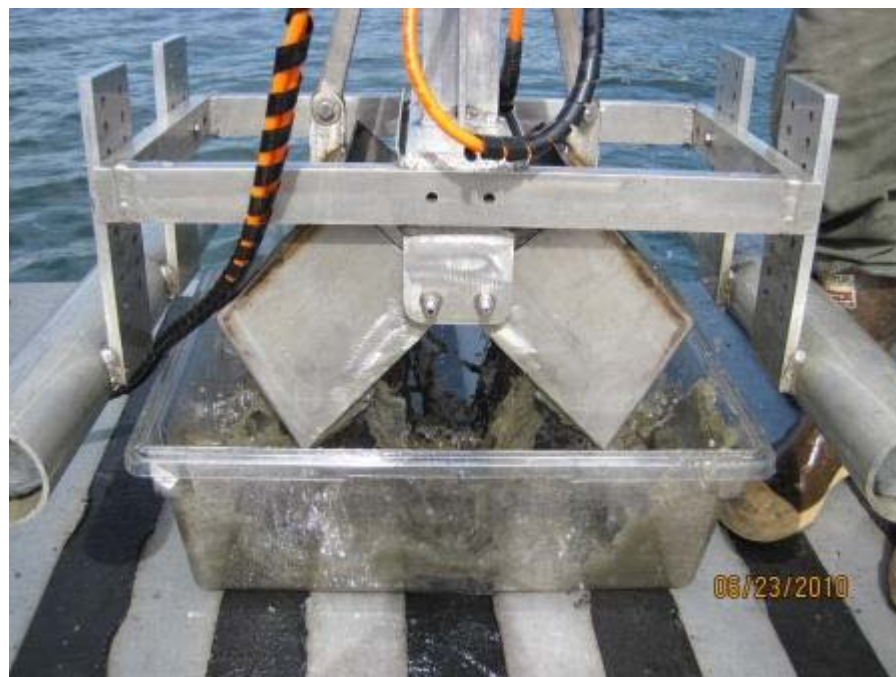
Release of sediment sample into Lexan tub
