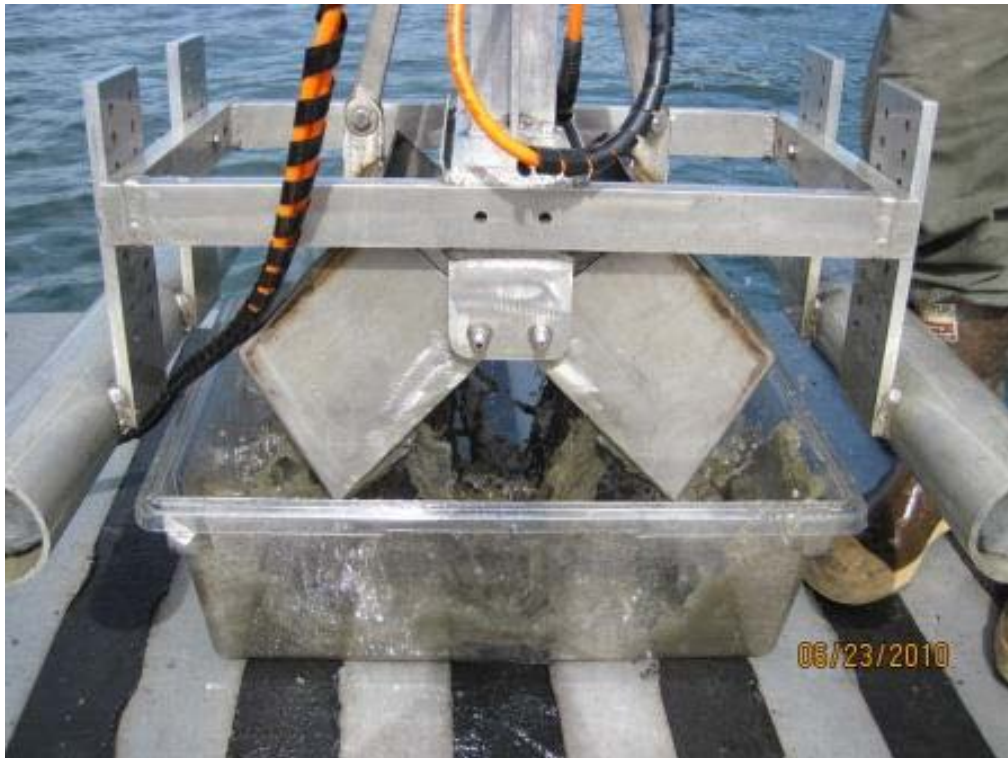
Photograph 3. Release of sediment sample into Lexan tub
