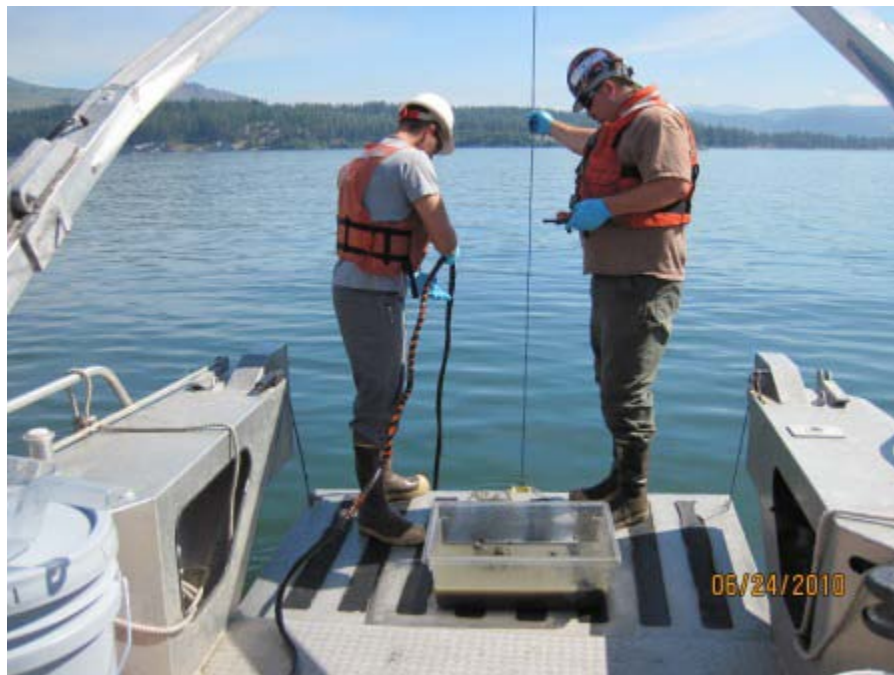
Power Grab Sampler on bottom and ready for pneumatic-actuation. Grab sample in Lexan tub.
