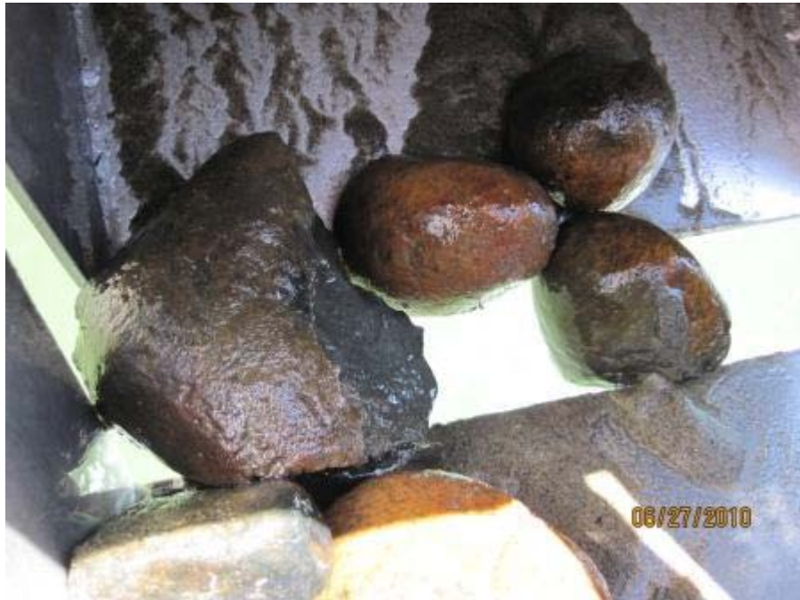
Cobbles and boulders with washing in sample aliquot attempt for unique sample identifier NP-03-004, sample rejected
