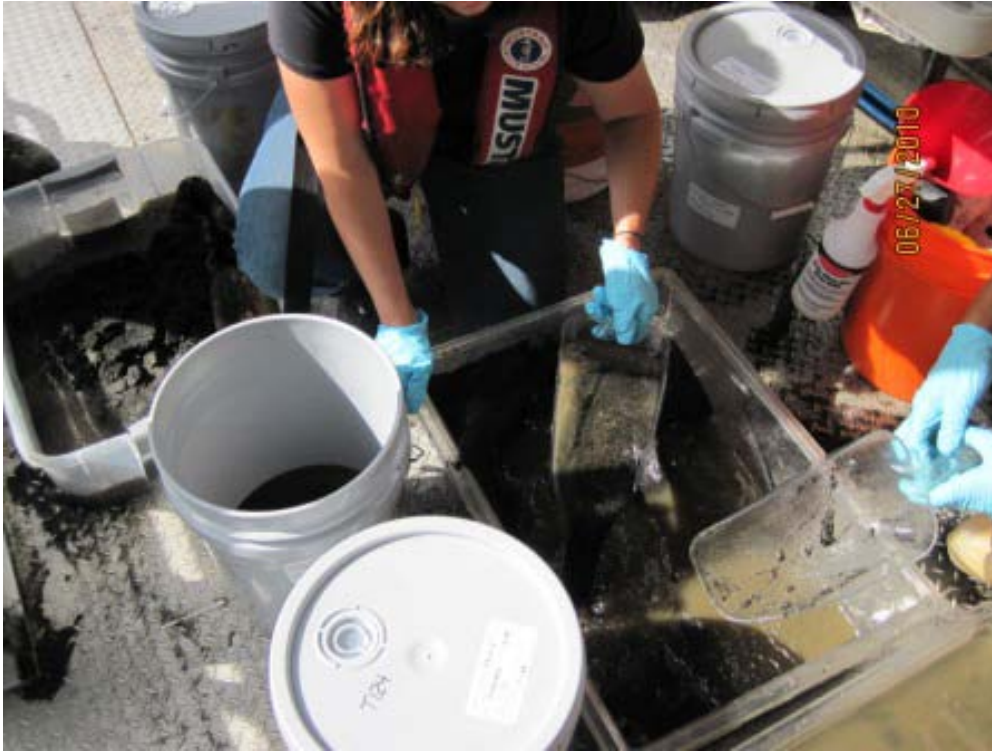
Photograph 4. Transferring sediment sample to decontaminated 5-gallon HDPE containers.
