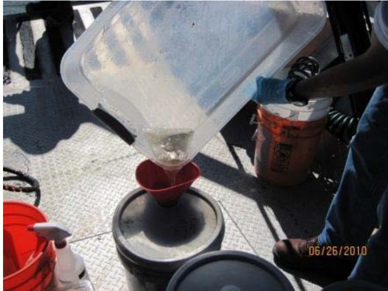
Collection of IDW into 5-gallon HDPE container
