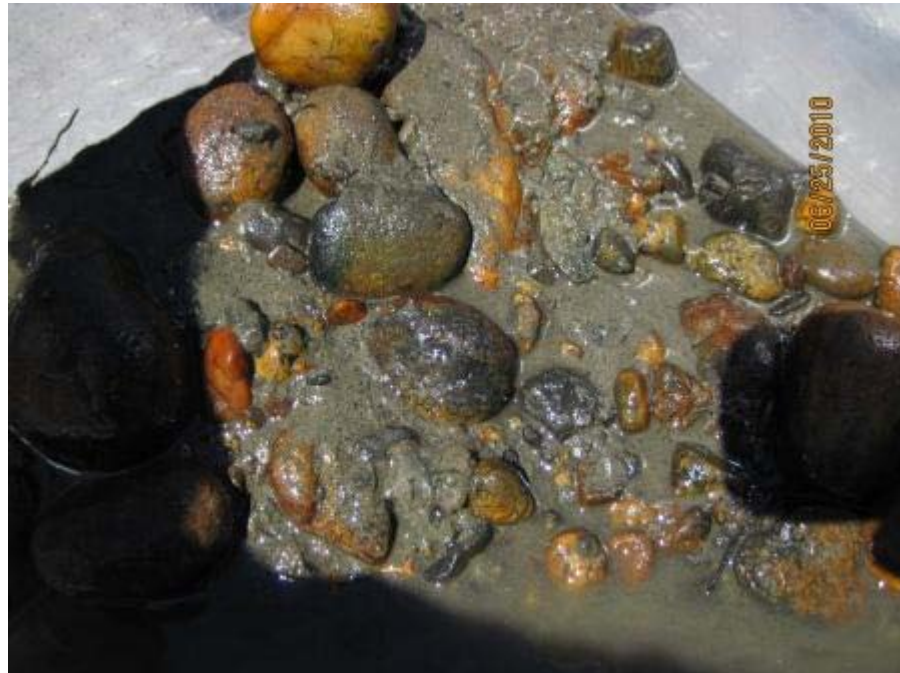
Sample washing and poor recovery at station CB-03, sample attempt rejected
