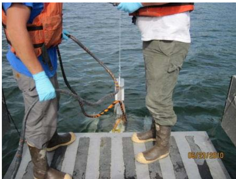
Lowering the Power Grab Sampler for sediment sampling
