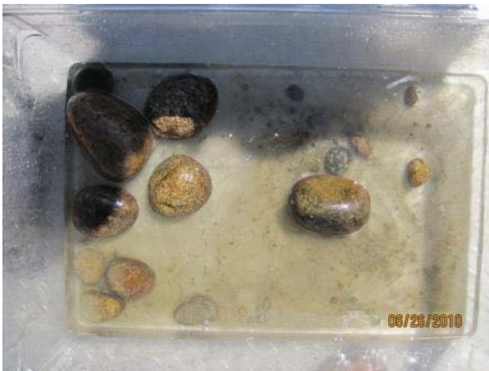
Photograph 7. Gravel and cobble sample at station DME-02; sample attempt rejected.
