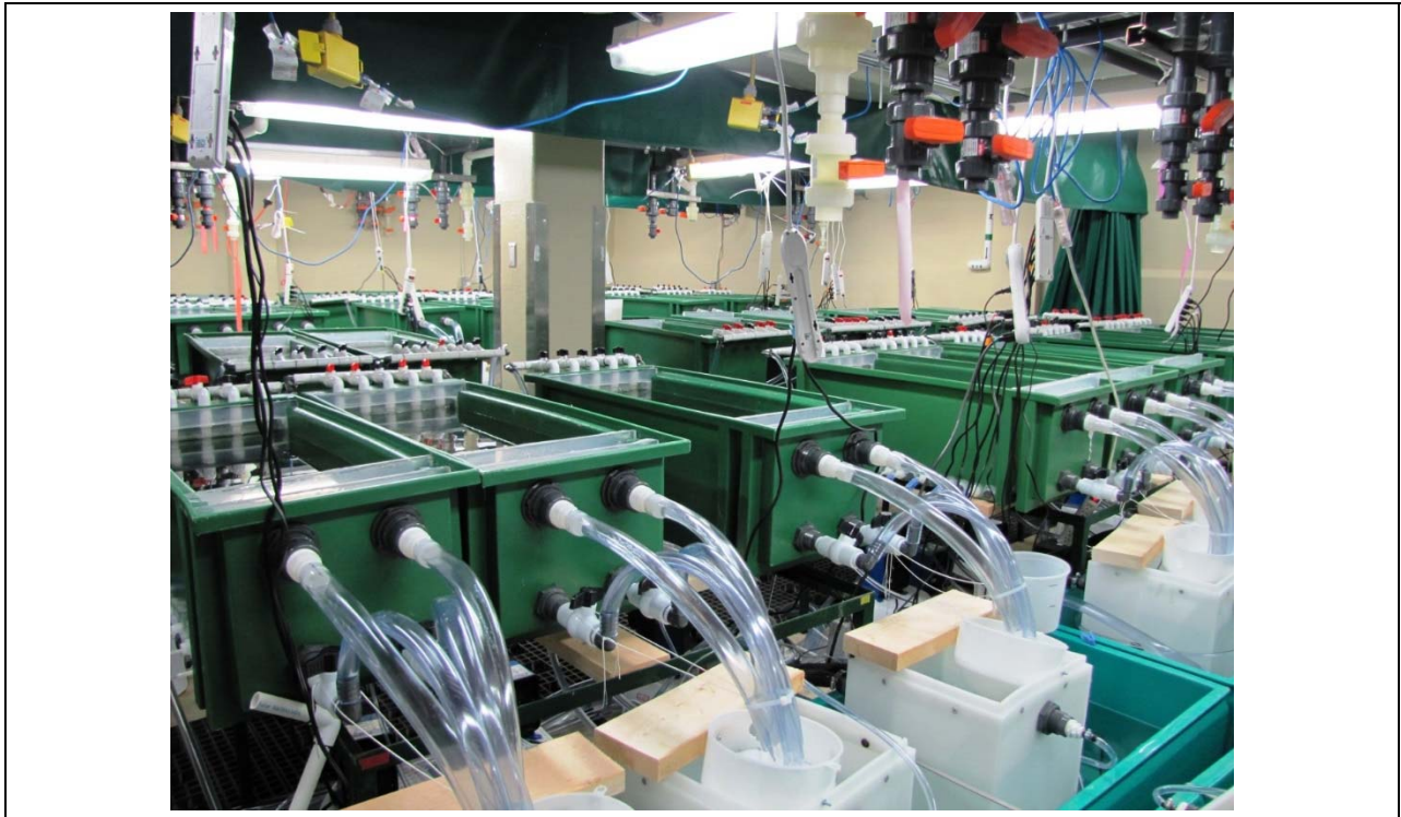
Photo D-2. White sturgeon sediment toxicity test exposure chambers as set-up at the University of Saskatchewan, Aquatic Toxicity Research Facility. Each green tub represents an exposure chamber.
