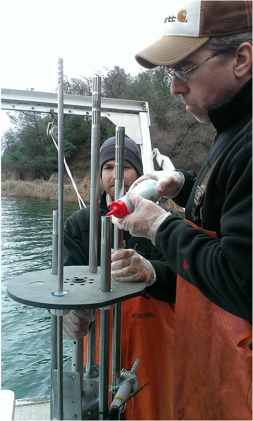
Figure 5. Multi-probe Trident porewater sampler setup with glass bead pre-filter system.
