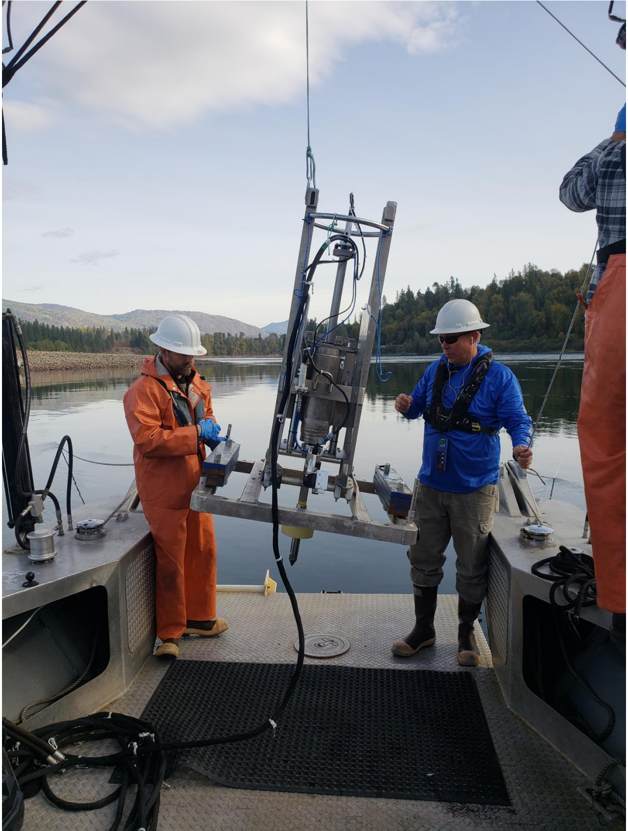
Figure 9. Trident Drive-Frame system installation.
