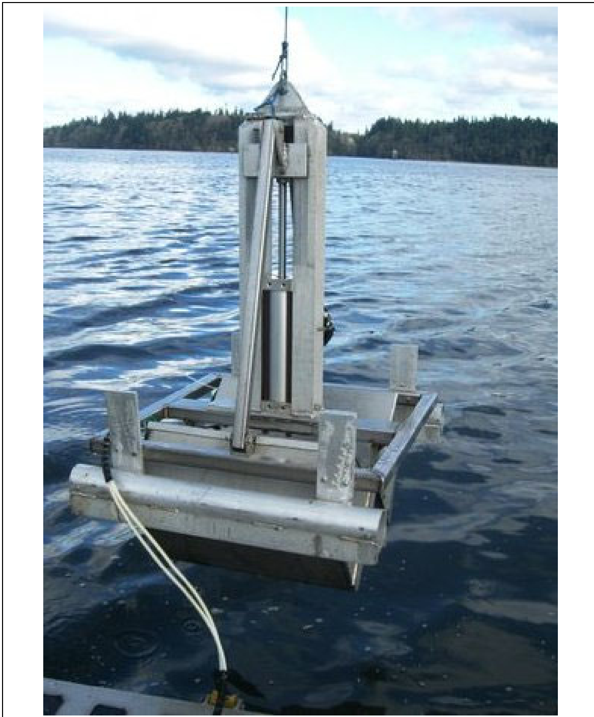
Figure 1. Illustration of Custom-designed Van Veen Power Grab Sampler
